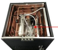
Drain water bath by removing white overflow pipe stem. Water will drain through drain line to drain.
