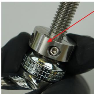
Place back half of the pivot ball mounting clamp over the collar on the back of the pivot ball.
