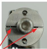
Secure with the rear clamp to the front clamp using the supplied 4-40 x 3/8" socket head screws. Secure the screw evenly and tighten firmly using the supplied 3/32 Allen wrench.
