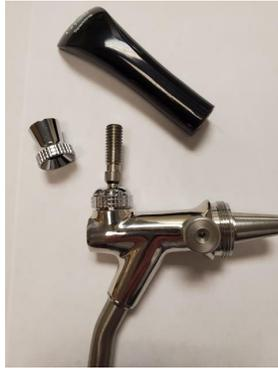
Lever comes assembled. It will need to be disassembled to install.
