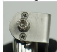
Secure the lever bracket to the mounting clamp using the two provided 4-40 x 3/8" Phillips, flat head screws and tighten firmly.
