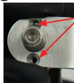
Place the lever over the top of the threaded pivot ball and align the holes with the tapped holes of the mounting clamp.
