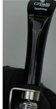
Next screw the tap marker onto the threaded pivot ball all the way down to the jam nut. Then back the tap marker off, aligning it with the front of the faucet. Once aligned, back the jam nut up into the bottom of the tap marker. Hand tighten the jam nut firmly into the tap marker.
