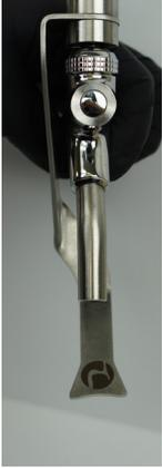
You may have to align the activation lever with the tip of the nozzle by slightly bending the bracket. Gently press or pull on the flat section of the lever where it is labeled "Crysalli".
