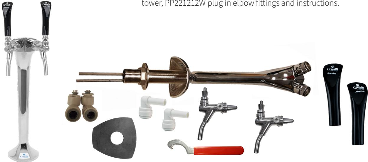
**Step 2:** Insert tower into the hole in the countertop for it, thread on and tightened the set nut to secure tower. Locate grey SI030812S superseal union elbow fittings supplied with the tower (one per tube). Loosen the collet nut on the fitting to the last thread then push the fitting onto the 1/4" stainless steel tube as shown on John Guest instruction page. Tighten the collet nut all the way down to lock fitting onto SS tube (failure to tighten the collet nut
