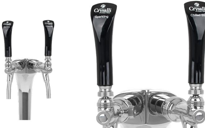
Once the faucet bodies are attached to the tower, thread the handles on to the them. Thread down until the position the handle with curve is facing you, if loose, tighten the black set nut up to the handle base to lock the handle in position. Apply the round sparkling and still water image stickers to the appropriate handles at the top of them.
