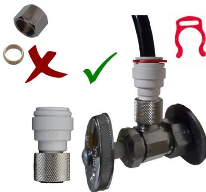
Locate the PSEI6012U9 angle stop adaptor in the UCM Install Kit. Locate the angle stop water source feeding the system, remove the compression nut and ferule ring from it and replace with the PSEI6012U9 fitting.
