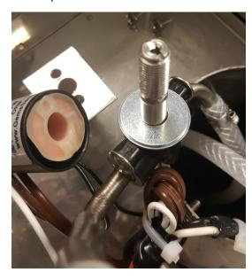
Remove the solenoid washer and Unscrew the Armature Stem from the valve body.
