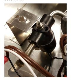
Turn valve over, being careful not to pull the wires from the solenoid.
