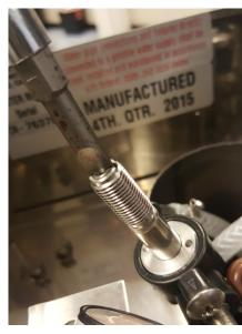
Watch for the Piston and Spring in the Armature Stem when removing it. Check that the spring has tension still and look the bottom of the piston over for debris and wipe clean.
