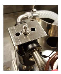
Lightly bend bracket to clear the adjustment nut and remove valve assembly.
