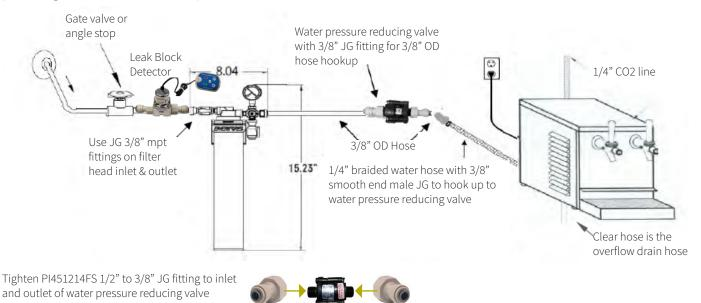
Optional accessory avaliable: CR-LD38JG Inline Leak Detector and Auto Water Shutoff.
