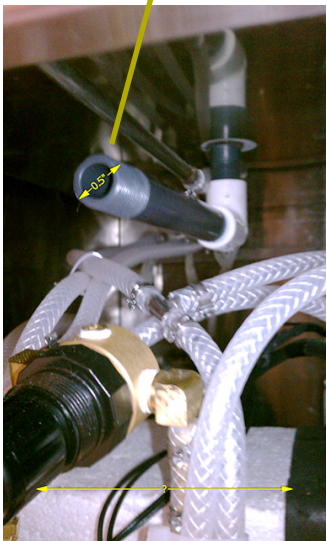
1/2" Ice bin drain fitting. Located in the back on the bottom of the bin.
