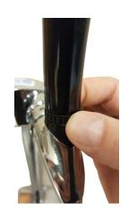
Once the faucet bodies are attached to the tower, thread the handles on to the them. Thread down until the position the handle with curve is facing you, if loose, tighten the black set nut up to the handle base to lock the handle in position. Apply the round sparkling and still water image stickers to the appropriate handles at the top of them.
