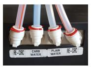
**Step 5:** If you are comfortable your connections are leak-free, wrap the exposed hoses and fittings with the insulated tape and push the unit in place.
