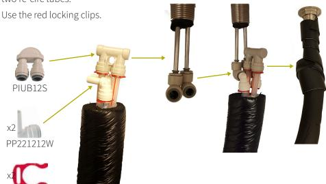
Step 4: Once assembled, connect the stem end of the plug in elbow fittings to the super seal fittings on the tower. Connect the blue striped tube to left faucet tube for sparkling water. Natural to still chilled water. If using a 3-valve tower, run a separate hose from the filter to the 3rd tube for ambient water. After testing the system for leaks, wrap all exposed hoses and fittings with the insulated tap found in the UCM install kit.
