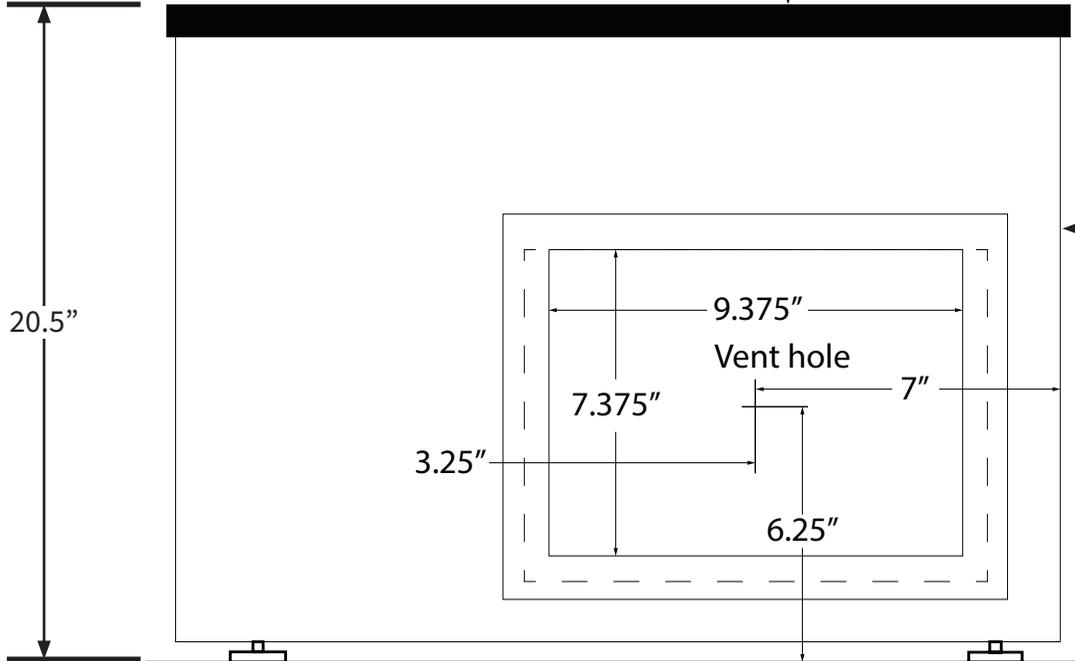
Allow a minimum of 4" clearance on one side of the chiller and the rear
