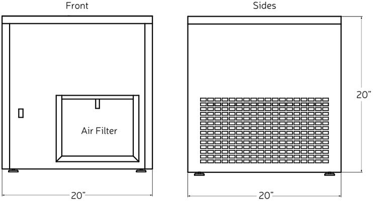
8" Allow 8" of clearance above chiller to remove lid and access water bath
