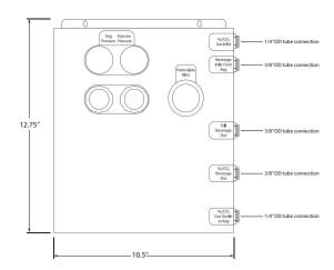
Enlarged view of iN2-2P injector
