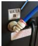
1/4" Braided Hose: CO2 w/ Flare nut Clear Hose: Overflow bath drain
